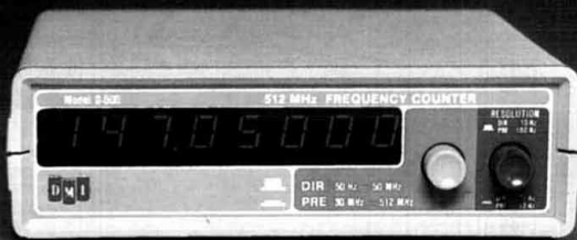
50 Hz to 512 MHz 1 PPM ACCURACY TCXO 5¼ X 5 X 1½
